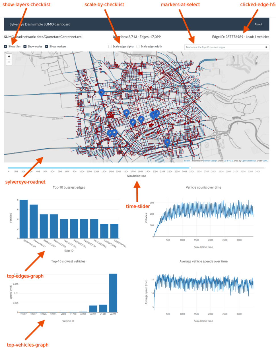
FIGURE 11. Layout of the dashboard made with Dash and the Dash Sylvereye library for analyzing a SUMO traffic simulation. Labels in orange are the Dash component identifiers referred to in Fig. 12.
