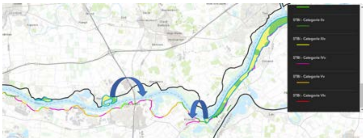
Figure 4. A first prototype of an ArcGIS Online web application linking soil excavation sites with dike sectors in the River Waal
