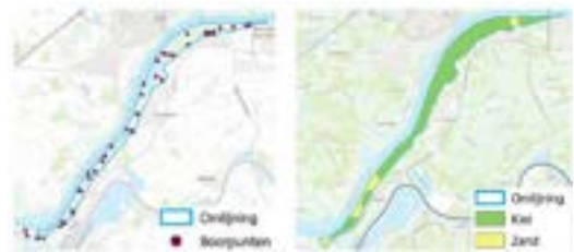
Figure 3. One of the proposed areas of excavation within the floodplain of the River Waal showing the clay deposits from the surface to a depth of 0.5 m.
