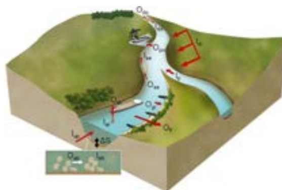
Figure 1. Representation of a channel sediment budget in a human-controlled river system, showing different sediment inputs (I), outputs (O) and the storage term ( \Delta S ). Source: Frings et al. (2019).
