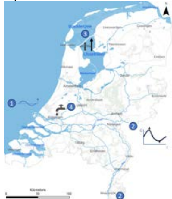
Figure 1. Main water system in the Netherlands with a schematic representation of possible impacts of climate change on the main water system. (1) Sea level rise, (2) more extreme discharges, (3) adaptive weir management Lake IJssel, (4) increased (fresh) water demand. Background image adapted from PDOK (2023).
