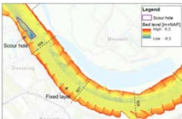
Figure 1. Bathymetry of the Waal near the side channel at Hurwenen (Source: RWS GeoWeb 12-06-2023).
