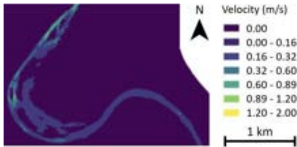
Figure 2. Excerpt of the model domain with flow velocities during low discharge conditions (around 20 m 3 s -1 ).
