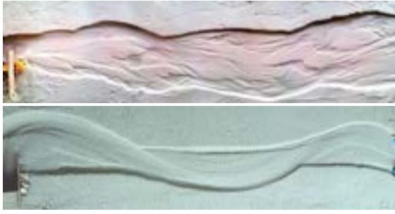
Figure 1. Channel development from straight in the laboratory with two different sediments: uniform sand (top) and poorly sorted sand behaving as cohesive at the flume scale (down).
