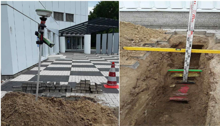
Fig. 8. Use of digital GNSS technology (left side) and analogue measures (right side) to determine utility locations.
