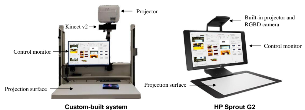
Figure 2. System illustration of custom-built PPM system on the left and the HP Sprout Pro G2 multimedia system on the right.
