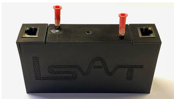
Figure 8: Second generation sensor with integrated differential amplifiers
