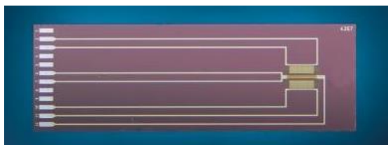
Figure 2. Flow sensor element with the heater in the center and two thermopile elements symmetrically arranged above and below the heater. The size of the entire chip is 6 mm x 2 mm.
