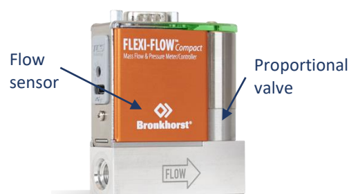
Figure 1. Example of an electronic gas flow controller. Photo courtesy of Bronkhorst.
