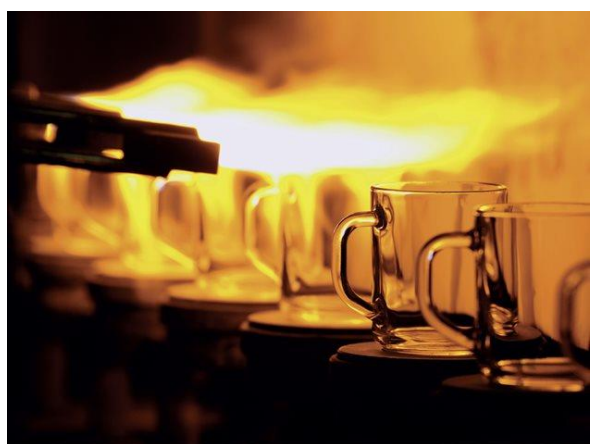
Figure 4. Gas flow control in burner applications for glass manufacturing. Fast ratio control of gases within the mixture results in a consistent flame temperature. Photo courtesy of Bronkhorst.
