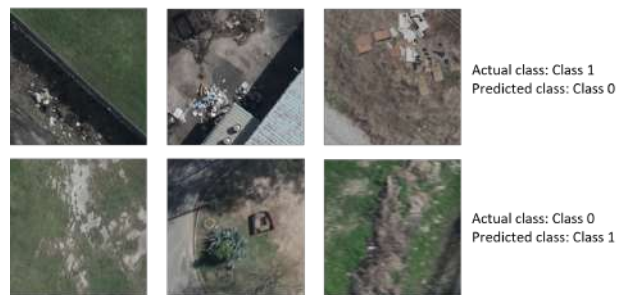
Fig. 5. Examples of false predictions of the DL models. Row-1 shows examples of the non-dumping class misclassified as dumping site. Row-2 shows examples of the dumping class misclassified as a non-dumping site.
