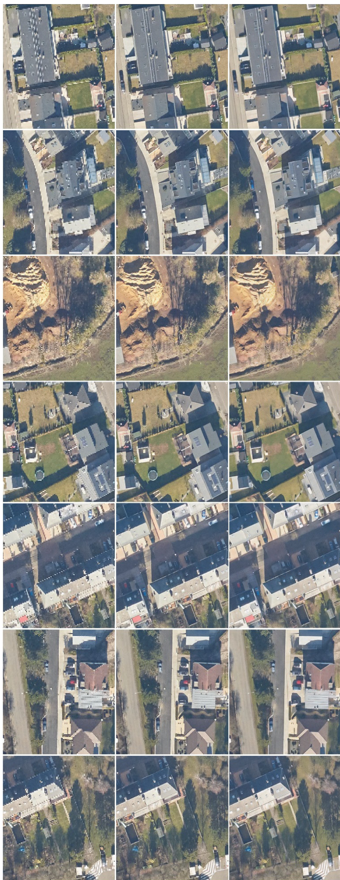
Fig. 4. SRR \times 4 results for the Luxembourg dataset. (Columns from left to right) LR, HR (ground truth), and SR images (inferred by our model).
