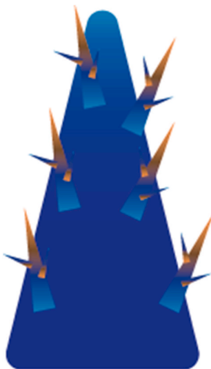
Fig. 10. A conical shape covered with smaller cones. The colour gradient on these smaller spines depict a wettability pattern.
