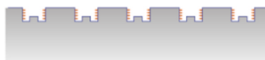
Fig. 12. Multilevel channels. The bottom of the main channel is covered with hydrophilic grooves and ridges (dark blue). The ridges are covered with hydrophobic structures (orange).
