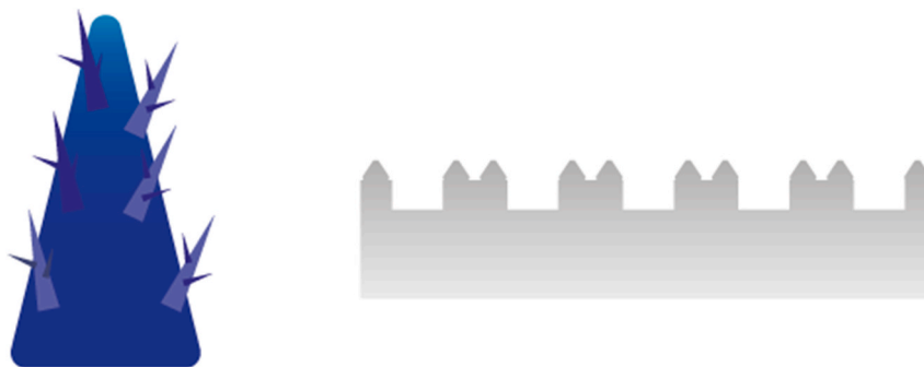
Fig. 4. Hierarchical structures for Moisture Harvesting; Micro-trees (left) and a more general hierarchical design consisting of grooves with spikes on top (right).
