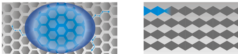
Fig. 9. Top view of a patterned surface resulting in a set of connected microchannels (left) and a top view of an asymmetrical channel structure (right).
