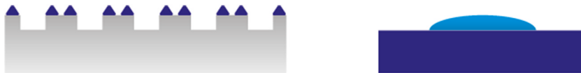
Fig. 7. From left to right: A biphilic surface with hydrophilic (dark blue) nano bumps on a (super)hydrophobic (grey) surface with micro scale grooves & a single hydrophilic substrate with a droplet on top (light blue).
