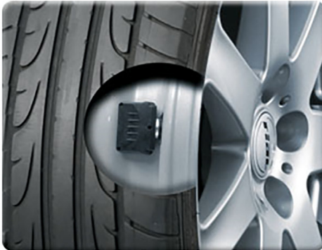
Figure 1 A TPMS device installed (a, b) at the lateral side of the rim and on the inner liner (c) [7].
