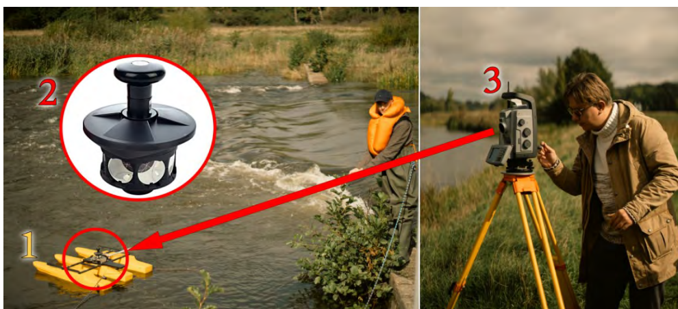
Fig. 2. Scheme of measuring stand. (1) Floating benchmark, (2) 360 prism, (3) precise total station.
