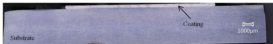
Fig. 6 Microscopic image of FSC experiment number 4. Clearly, no macroscopic mixing of coating and substrate occurred at the interface.
