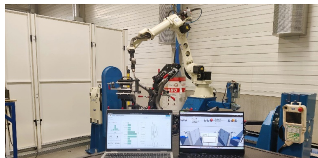
Figure 2: The welding robot and representations of its digital twin
