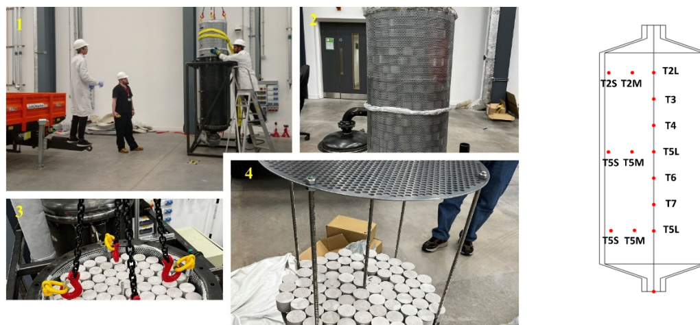
Figure 1. Right : 1: Stack of trays loaded in the tank; 2: Stack of trays inside a cylindrical aluminium sieve; 3: top of tank after loading the tray; 4: First pellets loaded on the bottom tray.; Left : Thermocouple positions in the tank.
