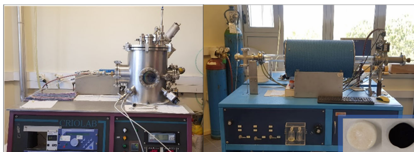
Figure 46. PVD (left) and CVD (right) devices (DEMaC facilities) and comparison of LiNaSO 4 pellets before and after the deposition process [4].
