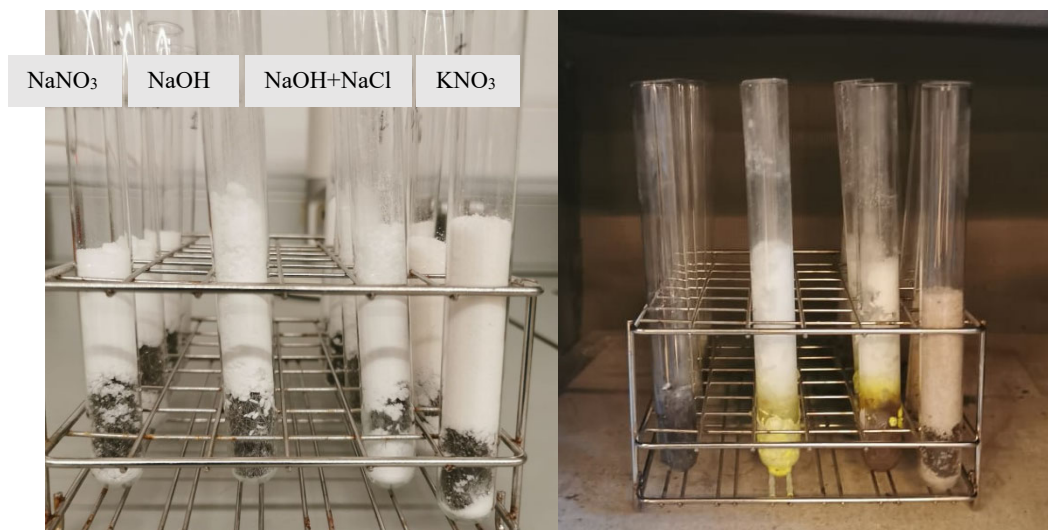
Figure 42. Immersion of stainless fibres in each PCM. Left: solid, right: liquid
