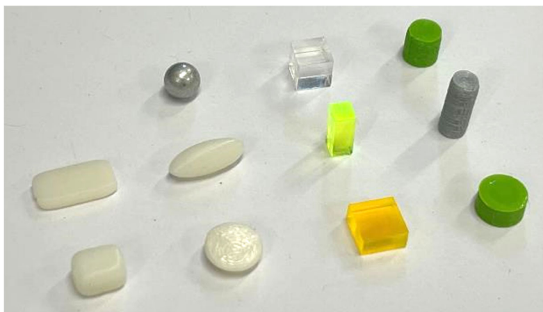
Figure 37. Overview of the produced particles, from top left to bottom right: Sphere, Cub_AR10, Cyl_AR10, SE01, Ell_AR25, Cub_AR25, Cyl_AR25, SE02, Ell_AR05, Cub_AR05, Cyl_AR05.
