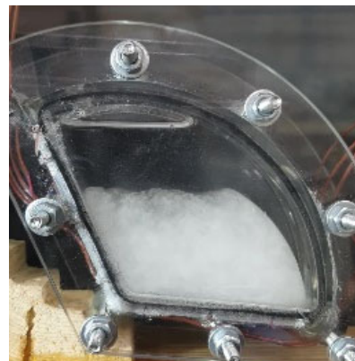
Figure 2. The experimental melting patterns for 30° (left column) and of 15° (right column).
