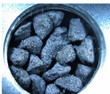
Figure 28. Potassium carbonate grains placed inside a ring in climate chamber. A sample image used for image processing.
