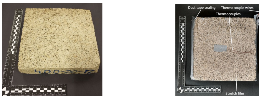
Fig. 1. The composite sample (left) and the prepared sample before the measurement (right).
