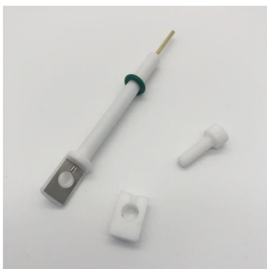
Figure A.1 b) Picture of Teflon electrode clamp purchased from AliExpress.
