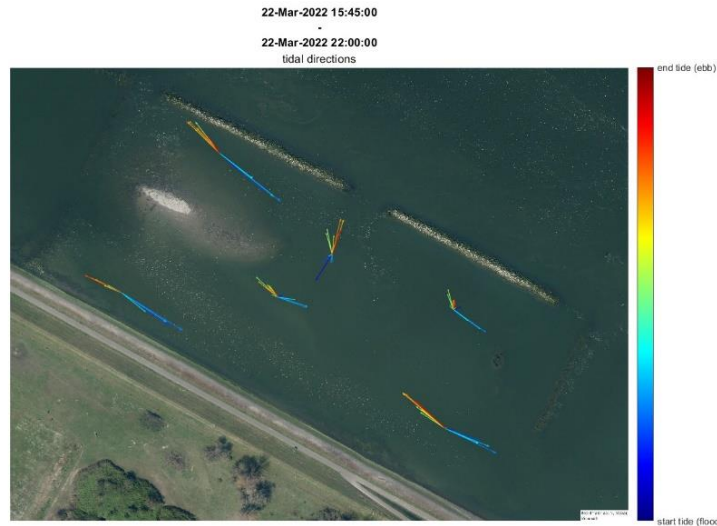
Figure 1: Flow directions during a tide. Start of the tide is marked in blue and is at low water before flood, the end is marked in red and is at the next low water at the end of ebb.
