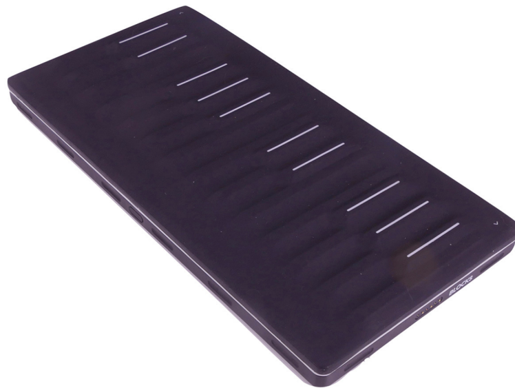
FIGURE 17 The ROLI seaboard MIDI input device used to record haptic touch patterns.
