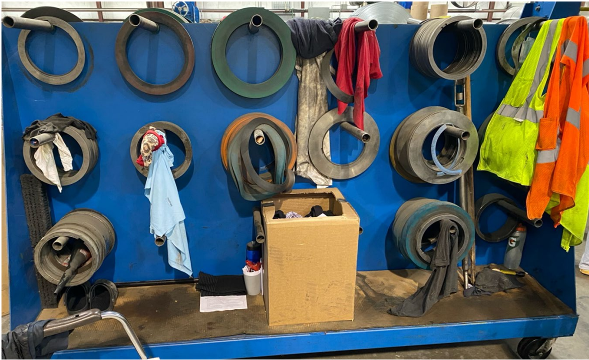
Figure 17: 60" slitter tooling storage rack.
