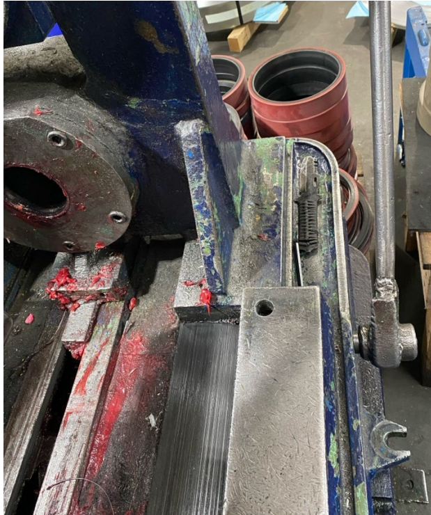
Figure 18: Grease build-up on a 48" slitter head.
