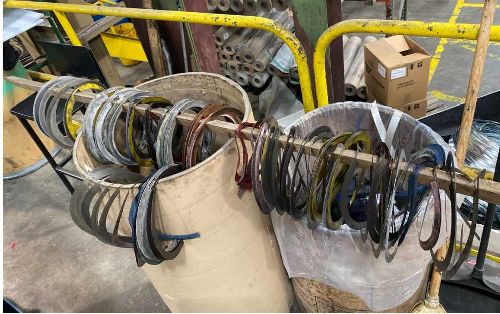
Figure 14: Wooden rod shim storage at the 60" slitter.
