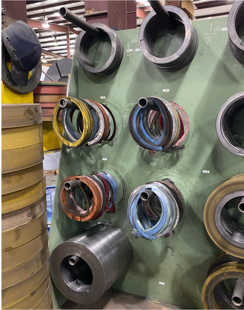
Figure 16: Rack hanging shim storage at the 60" slitter.
