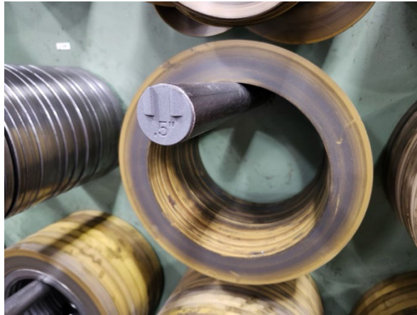
Figure 10: An endcap installed at the 60" slitter head-building station.
