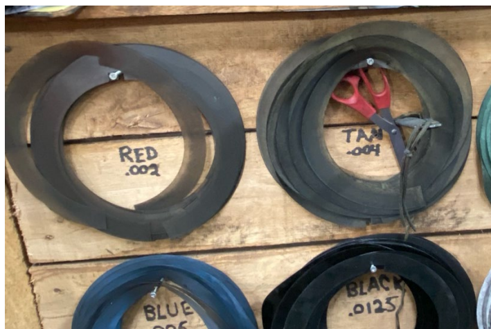
Figure 19: 48" slitter red and tan shims.
