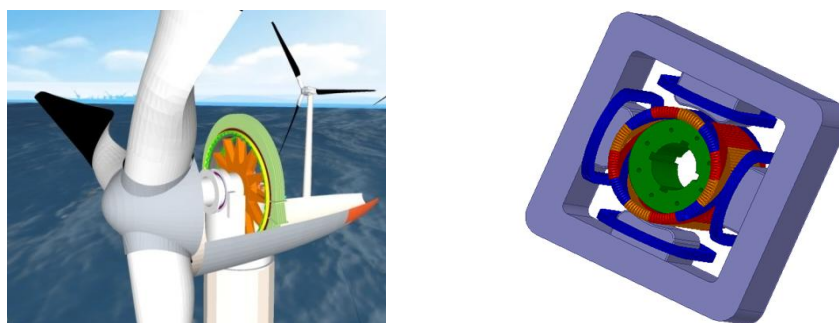
Figure 1. 10 MW superconducting generator concept (left) and 500 kW scale machine (right)
