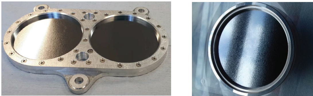
Figure 5. FSI Beamsplitter back-up solutions: (Left) Concept A Polypropylene beamsplitter, (Right) Concept B Mylar beamsplitter. (Courtesy of Cardiff University)
