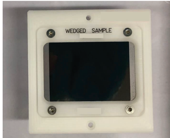
Figure 3. FSI interferometer full size wedged diamond beamsplitter breadboard uncoated (Left) and after Germanium coating (Right) - Concept B
