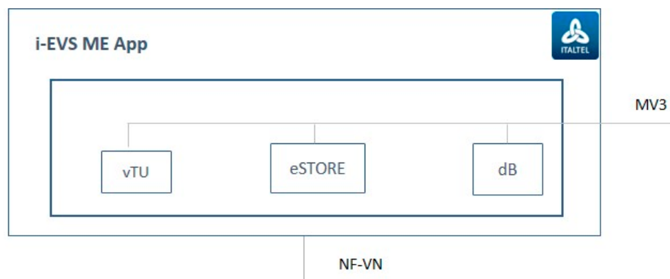
Figure 8. The i-EVS VNF architecture.
