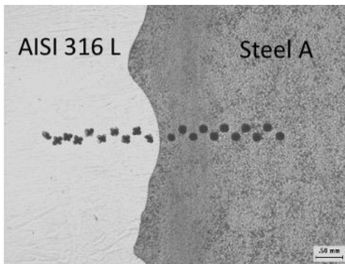
Fig. 5 Interface indentation through thickness profiles
