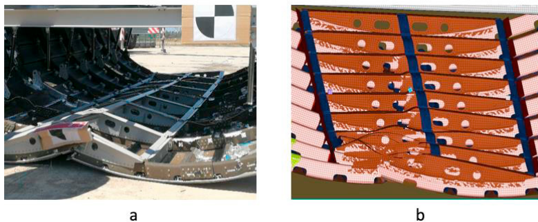
Fig. 10. (a) experimental vs. (b) numerical damages.
