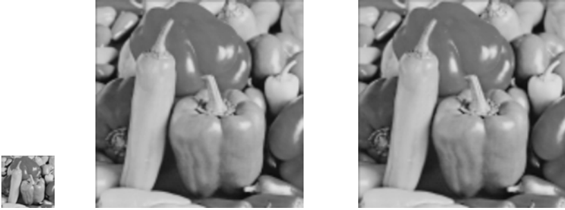
Fig. 4. The LR 128×128 input image, left, the 512×512 image reconstructed by bilinear interpolation, middle, and by the improved algorithm, right
