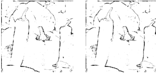
Fig. 6. The difference image for the peppers image obtained by bilinear interpolation, left, and by our improved algorithm, right
