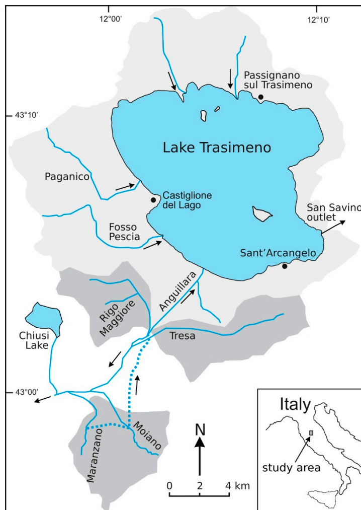
Figure 1. Location of the study area and main features of the Lake Trasimeno basin. The light grey area indicates the natural catchment of lake Trasimeno and the dark grey areas indicate the river basins artificially connected to the lake after 1957. The blue dotted line represents the artificial waterway connecting the Moiano and Maranzano river basins to the Anguillara channel.
