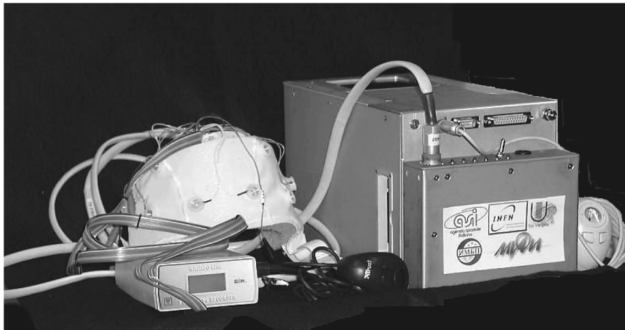
Fig. 1. Photo of the Sileye-3 detectors. Left: the EEG box and sensor caps. Right: the cosmic ray telescope. On the rightmost part it is possible to see the joystick for LF detection.
