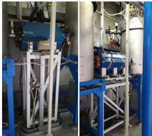
Figure 3: Photo of the old type of triplets (20 T/m, left) and the new one (30 T/m, right).
