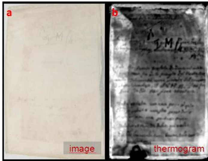
Fig. 1 - Photograph (a) of a seventeenth century volume. The thermogram (b) shows the writing of a leaf beneath the end paper
