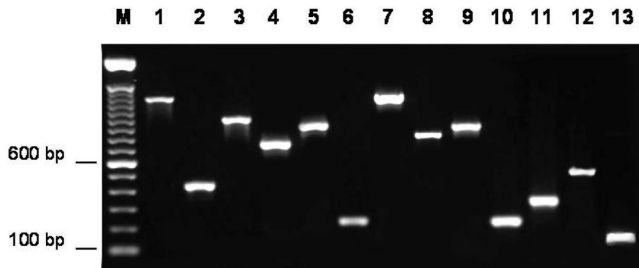
Fig. 2. Amplicons of the genes encoding staphylococcal virulence determinants and toxins genes. Lane M: DNA molecular weight, 100 bp. Lane 1: 23S rRNA. Lane 2: nuc . Lane 3: clfA . Lane 4: spa Ig-G binding 810 bp. Lane 5: spa Ig-G binding 970 bp. Lane 6: spa X-region. Lane 7: fnbA . Lane 8: fnbB . Lane 9: cap5 . Lane 10: sea . Lane 11: sed . Lane 12: seh . Lane 13: sej .
