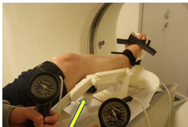
Figure 2 Porto dynamic MRI using a nonmetallic device.
