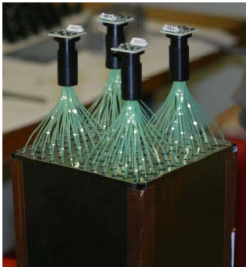
Figure 7: Fibre bundles with attached APD and preamplifier of four towers of an EMCAL module.
