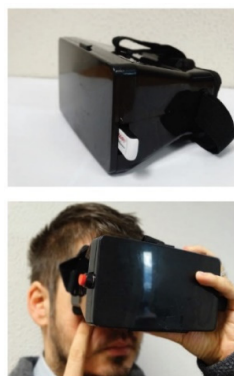
Figure 1. Device for acquiring the conjunctiva image.
