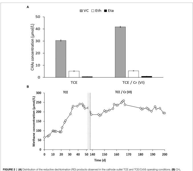
concentrations in the catholic effluent of the bioelectrochemical reactor during all the system's operation periods, including the runs with TCE and TCE/Cr(VI).
