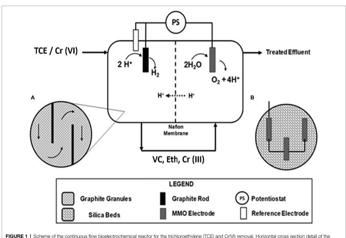
FIGURE 1 | Scheme of the continuous flow bioelectrochemical reactor for the trichloroethylene (TCE) and Cr(VI) removal. Horizontal cross section detail of the cathodic chamber (A) and schematic representation of the MMO (Magneto special Anodes, Netherland) electrode inserted in the silica bed (B).
