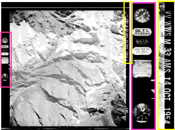
Figure 2. Example of scanned aerial image from 1954 over a glacial area together with zoomed views of the side information on the image.
