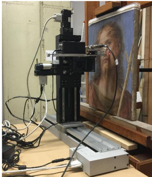
Figure 16. Acquisition of the data on the Gherardini artwork using the new THz imaging prototype.
