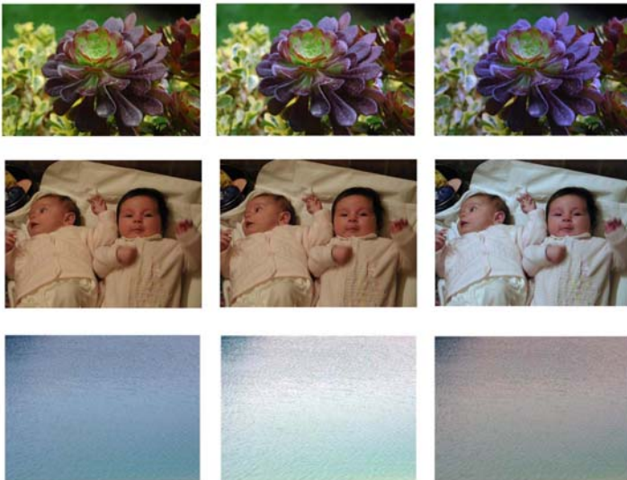
Fig. 1. Examples of different color corrections. First column: original images; second column: corresponding images processed by a white patch algorithm; third column corresponding images processed by a Gray World algorithm. Note that for certain images a do nothing strategy is preferred (for example for the image of the last row.)
