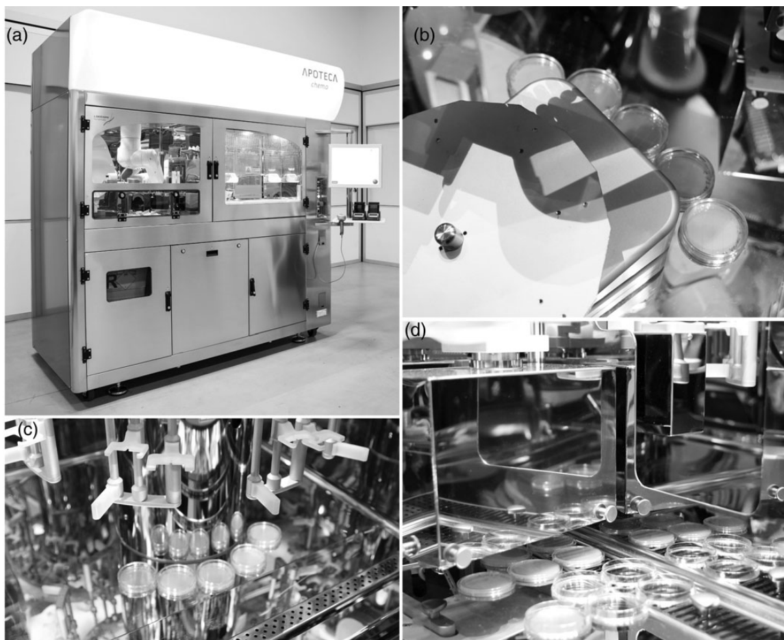
Figure 1 The APOTECA chemo robotic system (a). Plate location in the three shadow zones inside APOTECA chemo: (b) beneath the scale; (c) behind the vial stirrer; (d) around the internal warehouse.
