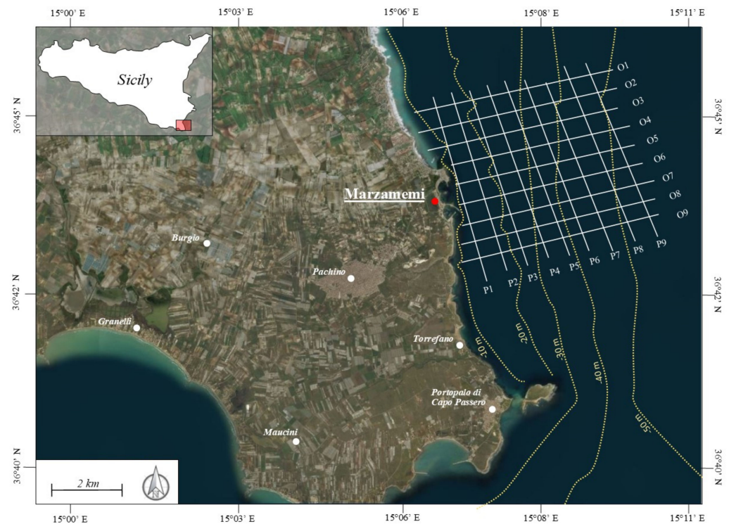
Figure 1. Geographic map (WGS 84) of the south-eastern Sicily and the offshore sector investigated in the present study (Marzamemi area). In yellow are the main bathymetric contours; in white are the locations of all seismic profiles.
