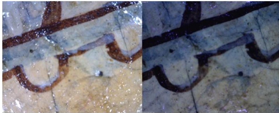
Fig. 14. A detail of figure 9; the fluorescence (on the right) of iron oxide, copper carbonate and calcium carbonate is shown
