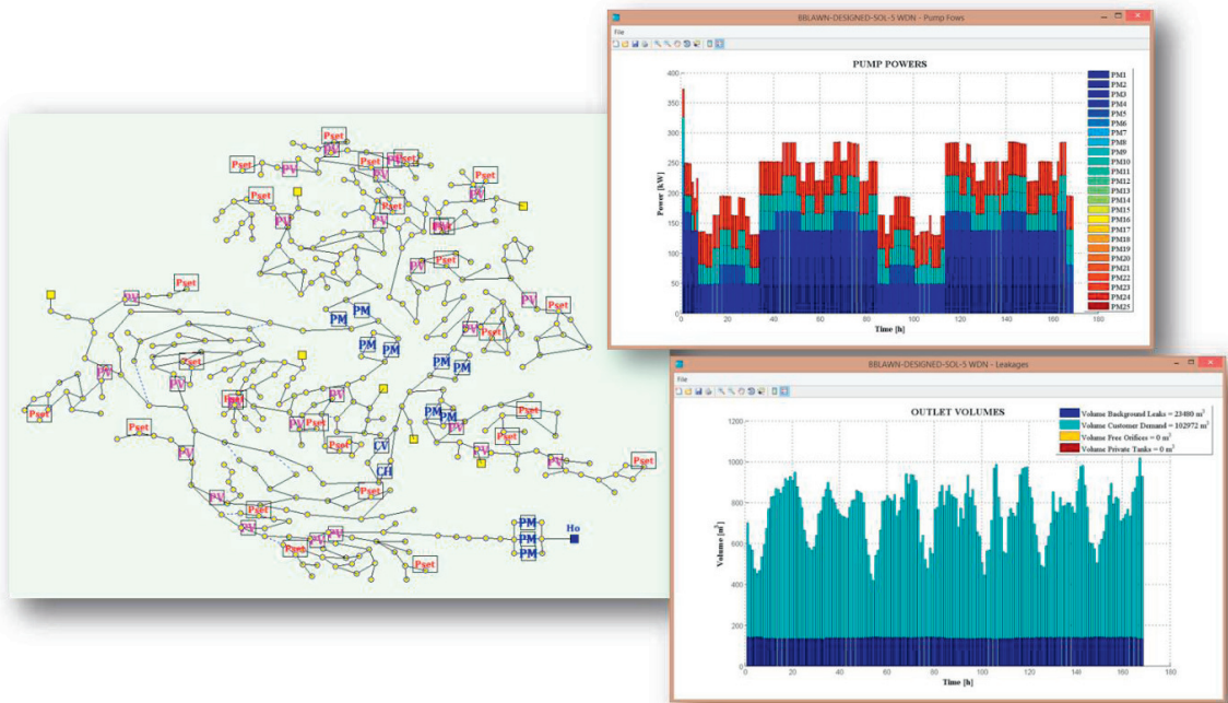
Fig. 2. Example of solution presented at the Battle of Background Leakage Assessment in Water Networks.
