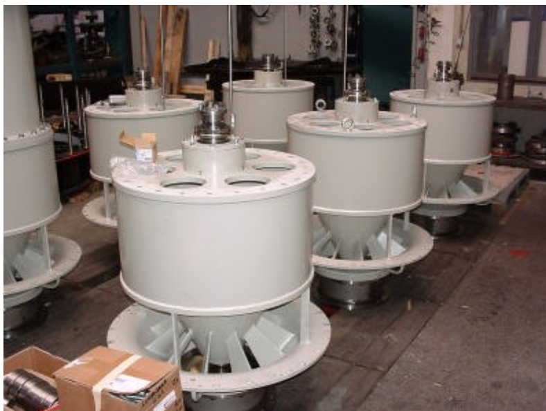
Figure 9: The six axial propeller turbines being assembled at Kössler GmbH (left) and one of the turbines being installed on the prototype in open sea
