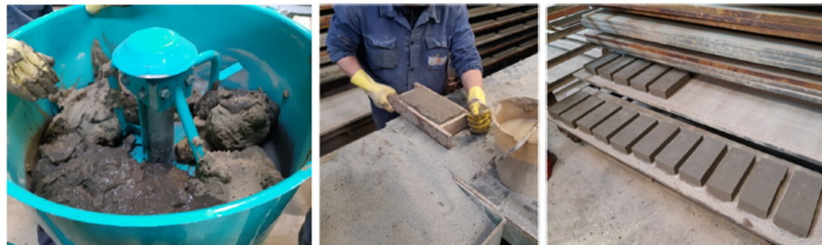
Figure 1. Main steps of brick manufacturing, from the left, preparation of DS and NC mixture, molding, and curing phase.
