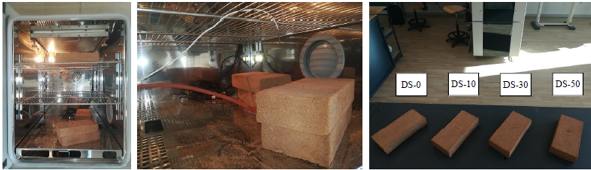
Figure 2. From the left, the climatic chamber apparatus, a detailed view of the hot disk measuring sensor, and an overview of the four brick specimens that were assessed.
