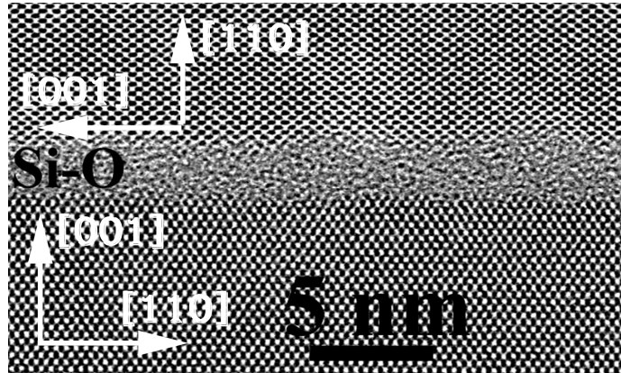
Fig. 2. Cross-sectional image of a Si(110)/Si(001) bonded structure after 15 min annealing at 1150 °C.
