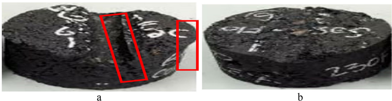
Fig. 2 Cracks in asphalt concrete samples of wheel tracking test a. stone dust sample and b. bagasse ash sample
