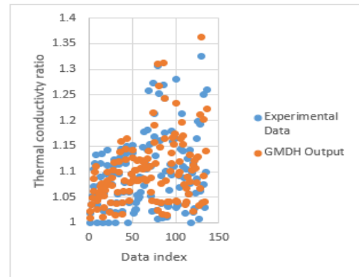
Figure 5. Comparison between experimental data and GMDH output for Al_2O_3 /water nanofluid
