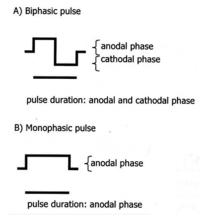
Fig. 1. Schematic of monophasic and biphasic pulse forms.
