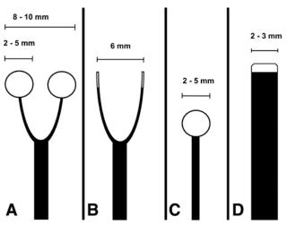
Fig. 2. Schematic of probes used for bipolar stimulation with ball tips (A) or straight tips (B) and for monopolar stimulations with a ball tip (C) or straight tip (D).
