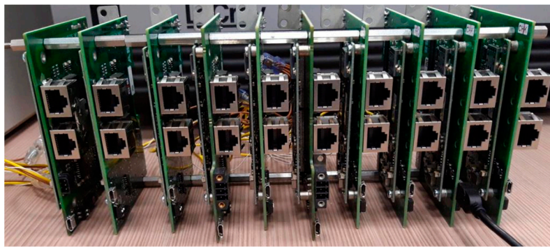
Figure 4. Experimental system setup: cluster of ten Power-One Italy S.p.A. a member of the FIMER Group inverters. Interconnections between inverters are not present.
