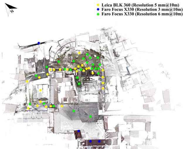
Figure 2: Positions of the X330 scans (green and blue) and the BLK360 scans (yellow)
