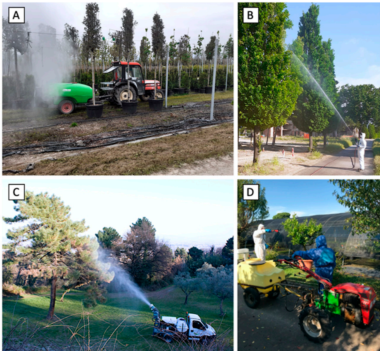
Figure 1. Conventional methods for pesticide distribution used in the ornamental plant sector. (A) A trailed agricultural atomiser (air-blast sprayer) used for potted or in soil trees or big shrubs; (B) a long-range spray gun commonly used for single trees or shrubs; (C) a centrifugal fan with long-range and wide-angle spray treatments commonly used for high trees; (D) a boom sprayer used for intra- and inter-row treatments, both in greenhouses and open-fields.
