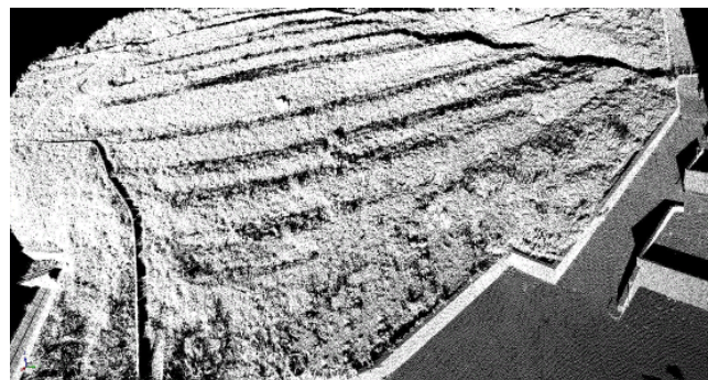
Fig. 6. Global cloud of points cleaned after the recording with LS3D of the scan at the time t_2 .
