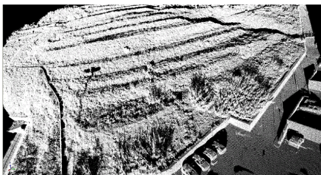
Fig. 5. Global cloud of points cleaned after the recording with LS3D of the scan at the time t_1 .
