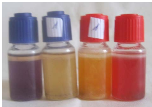
Figure 1. From left to right: Negative control vial for total viable count; positive total viable count vial; positive total Coliforms vial and negative control vial for total Coliforms.
